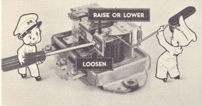
upper contact bracket as required. Make sure the points line up properly and tighten the screws well after adjustment.
