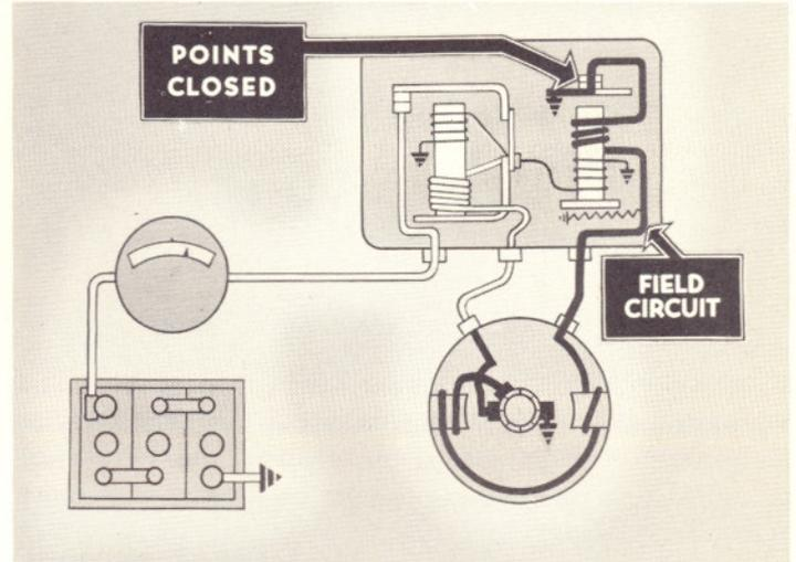
The voltage regulator, like the cutout relay, has two windings. The voltage, or shunt, winding carries full system voltage at all times. It is the working coil and does the work of attracting the armature. The field current or accelerator winding carries the generator field current directly to ground when the contact points of the regulator
