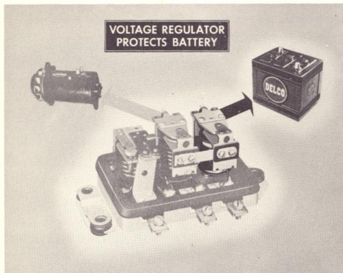
Since the cutout relay, the voltage regulator and the current regulator are mounted as one unit, it is advisable to check the entire generator regulator when any adjustment is required. A diagnosis or a system of "quick checks" readily determines whether or not the generator regulator does need adjustment, when some abnormal condition exists in the car electrical system.
