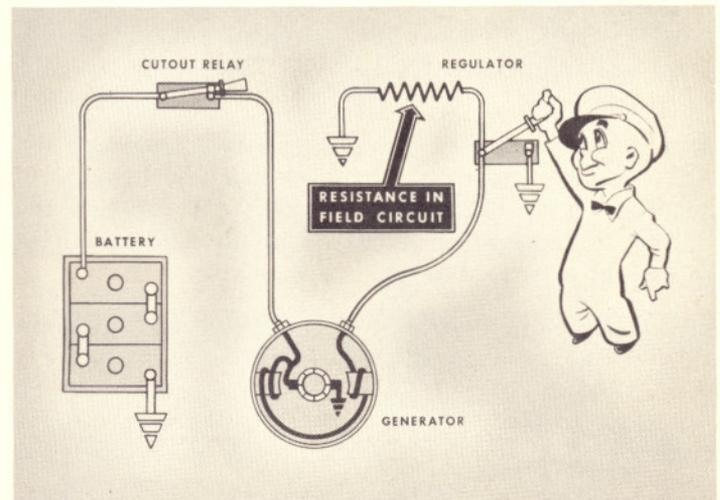
of generator voltage or current output is accomplished only by varying the strength of the generator magnetic field. Putting the required resistance in series with the field circuit at the right time is all that is needed to obtain satisfactory regulation. There are, of course, refinements in methods of changing the effective field resistance, which determine the excellence of the final results.
