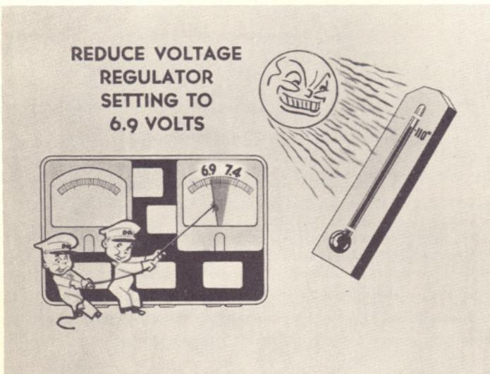
voltage regulator setting to as low as 6.9 volts in extreme cases instead of the specified 7.0 - 7.7 volts. The voltage should not be lowered for occasional trips as a normal setting would prove more satisfactory. When a reduction is made, care must be taken that the cutout relay closing voltage is approximately .5 volt lower than the voltage regulator.
