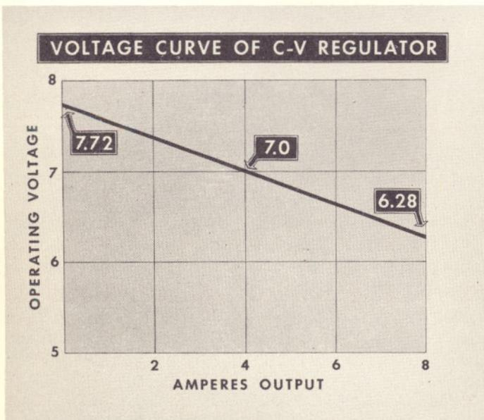
With Delco-Remy combined current-voltage regulators, tractor type batteries are giving better than average life because the charging rate even to a hot battery, with a properly set regulator, does not exceed a normal charging rate of approximately 1 ampere per positive plate per cell. It is also possible to get some charge to the battery in cold weather due to the higher voltage operation possible when the charging current is low.
