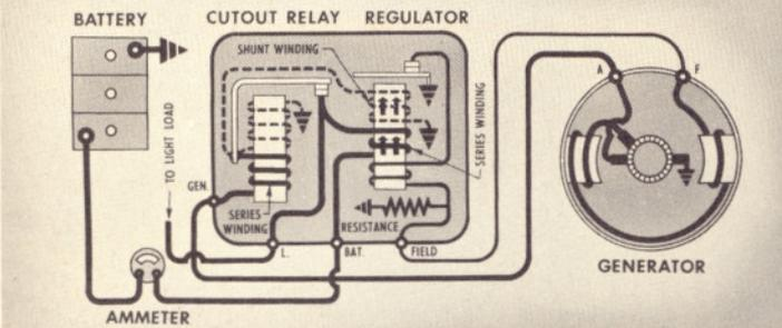
to lower the operating voltage. A high output is thus obtained only when the battery needs a charge, and the amount of charging current is controlled so that batteries are not subjected to overcharge, one of the main reasons for battery failures.
