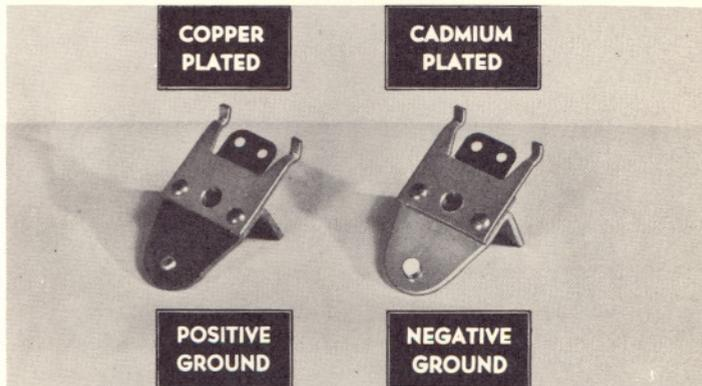
As a safeguard against installation of the wrong polarity regulator, the regulators designed for positive grounded systems have copper plated current and voltage regulator armatures, while the regulators for negative grounded systems have cadmium plated armatures. Late model regulators also have model, voltage, and polarity clearly stamped on the base of the regulator.
