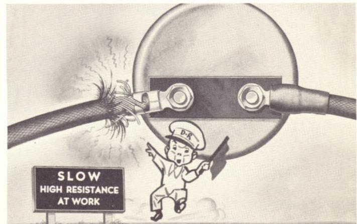
regulator will operate as if the battery were fully charged, even though the battery is in a discharged condition. A sulphated or defective battery may also be responsible for this condition.
