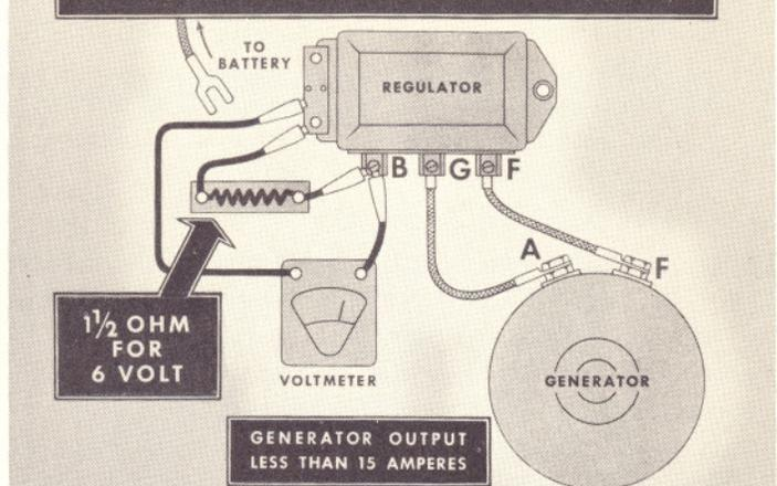
setting with the regulator at operating temperature and the generator running at a medium speed. The regulator cover must be in place. Cycle generator and repeat test.
