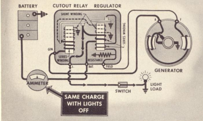
A feature of the combined current-voltage regulator is that generator output increases as the electrical load is added to the "L" terminal of the regulator. Since the load current by-passes the regulator current winding, it has no effect on the battery charging rate as long as the total load does not exceed the maximum output of the generator at operating speed.
