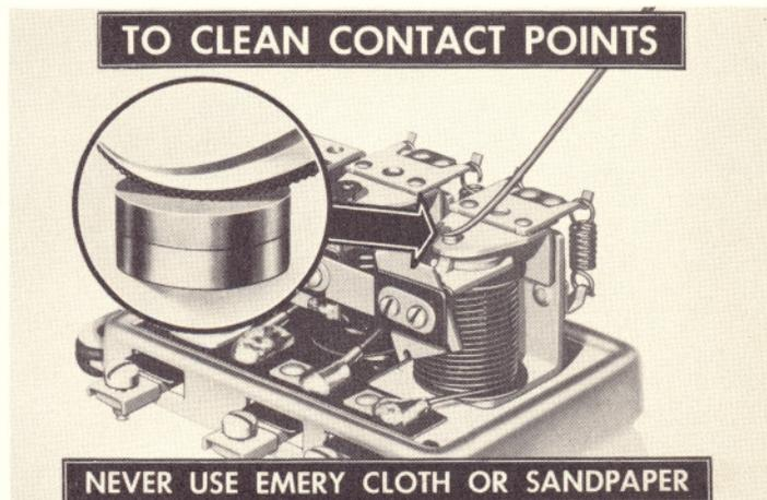
Emery cloth or sandpaper should never be used to clean contact points, since particles of emery or sand may embed in the contacts and prevent normal operation.
