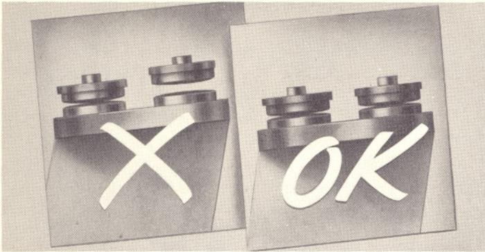
the two adjusting screws and raise or lower the armature as required. Tighten screws well after adjustment is completed.
