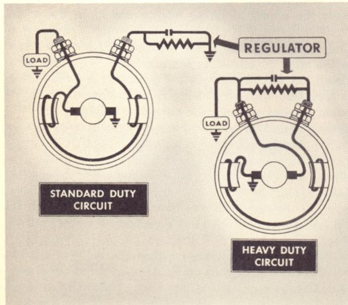
two types is in the method of connecting the regulator into the field circuit. In the standard duty type generator regulators, the generator field circuit is traced from the insulated brush through the field coils, then through the regulator and grounded at the regulator base. In the heavy duty type generator regulators, the generator field circuit is traced from the insulated brush through the regulator, then through the generator field coils and grounded inside the generator.
