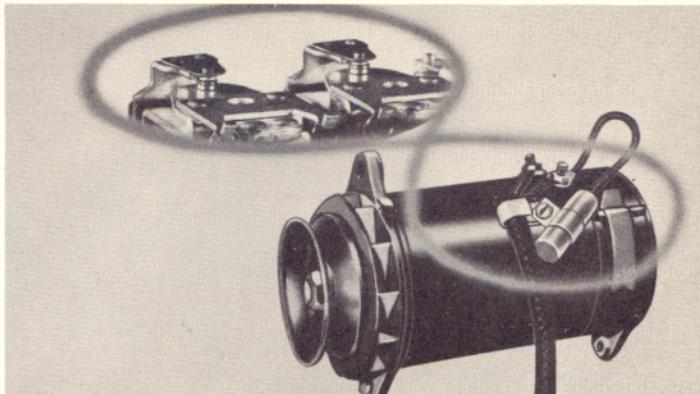
On the current and voltage regulator, pitted contact points will result from the installation of a radio by-pass condenser on the field terminal of the regulator or generator or from using the wrong model regulator for the application. Each model regulator is designed to operate with a particular model generator and a definite polarity system. Regulators must never be interchanged unless one model is actually superseded in the catalog by another.
