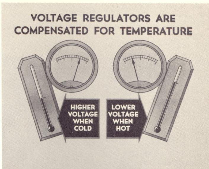
ture down would require a high voltage on a voltage sensitive winding and this is not desirable. Delco-Remy regulators are compensated for this temperature effect by means of a bi-metal thermostatic hinge on the armature.
