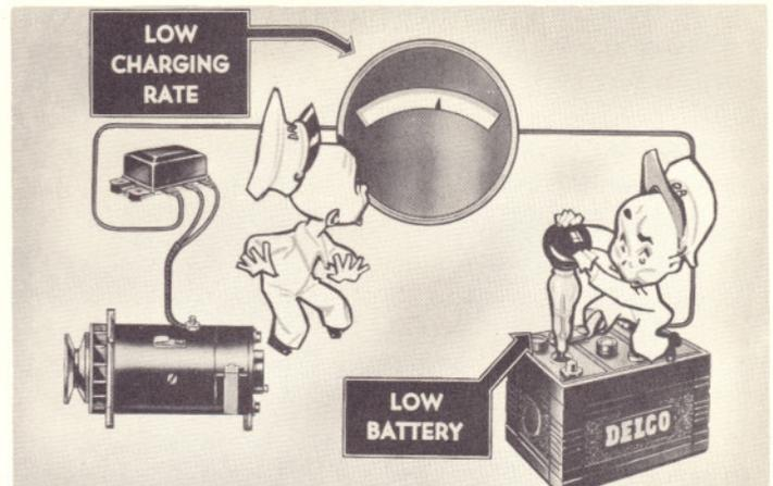
defective leads, loose connections at the ammeter or other junction points which cause high resistance in the charging circuit. When high resistance is present, the voltage
