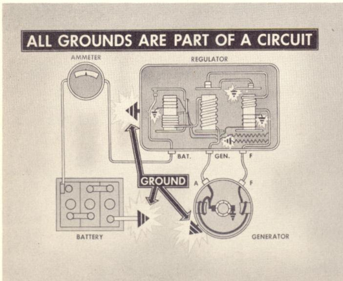
before reinstalling the regulator. The ground connections at the generator, regulator and battery are as much a part of the circuit as the wiring. Be sure a good ground exists at these units.
