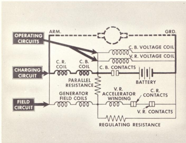
The voltage winding is the working coil and does most of the work in attracting the armature. With the points closed, the circuit between the generator and the battery is complete. Current flowing from the generator to the battery passes through the current winding of the relay in the right direction to add to the magnetism holding the points closed.
