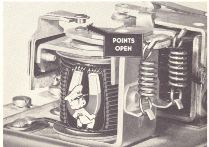
are held closed by spring tension. As the battery approaches a charged condition the system voltage increases, and the two windings build up sufficient magnetic strength to overcome the spring tension and separate the points. When the points open, the generator field current must flow through a resistance to ground, and this causes the generator output to drop off. The instant the points open, current stops flowing through the field current winding
