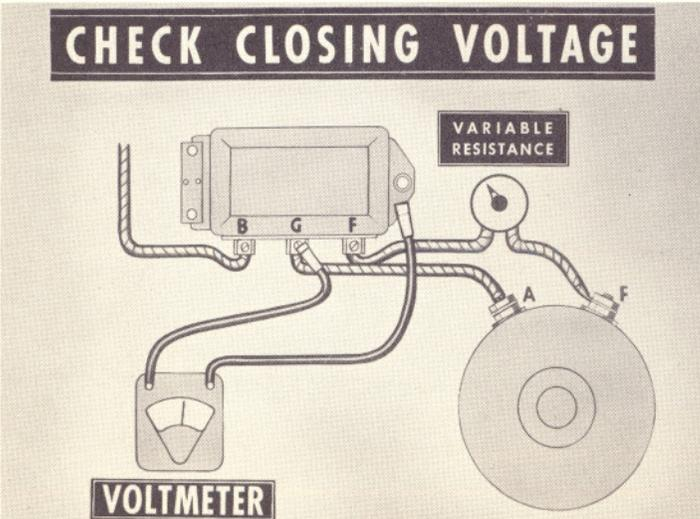
at medium speed. Slowly decreasing the resistance until the relay contact points close will also give the closing voltage setting.)
