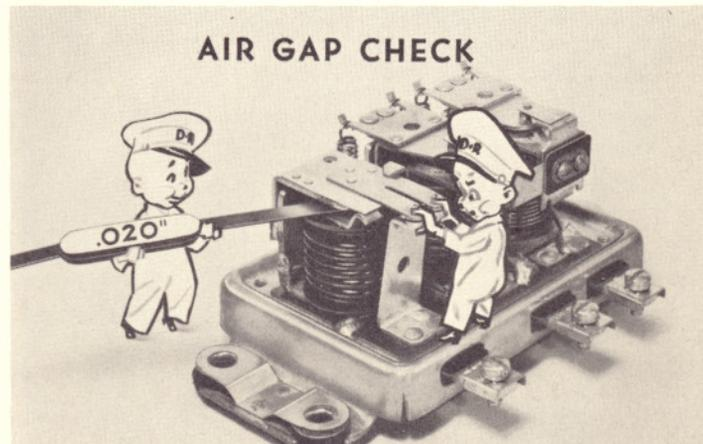
sets of points do not meet at the same instant, bend the spring fingers until they do. To adjust the air gap, loosen
