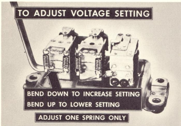
Operate the generator at specified speed. Adjust the spring tension so that regulator operates at 2/3 of the specified setting. Connect the voltmeter and fixed resistance from the battery terminal to ground, and complete adjustment on second spring to specified voltage without again touching the first spring. This procedure insures that each spring will carry one-half the total tension.
