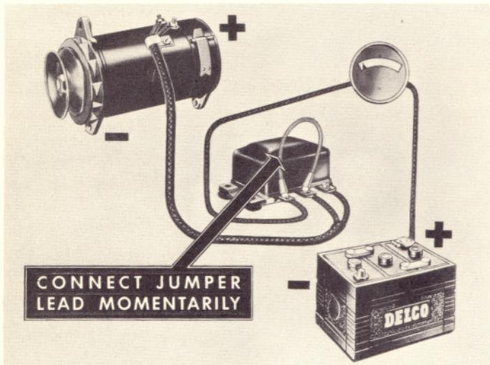
After any check or adjustment of the regulator or generator, particularly after leads have been disconnected and then reconnected, a jumper lead must be connected momentarily between the "BAT" and "GEN" terminals of the regulator, *before the engine is started*. This causes a momentary surge of current to the generator which correctly polarizes it with respect to the battery. This
