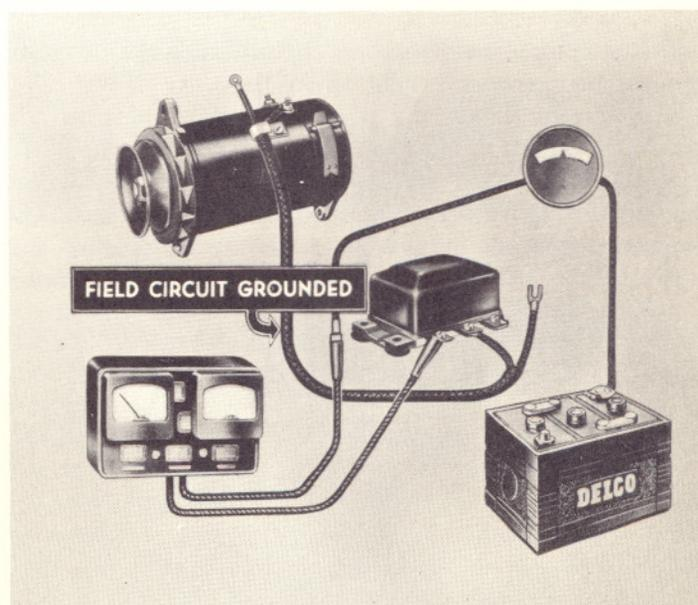
the output does not drop off under either of these checks, the generator is at fault and should be removed from the engine for further check.
