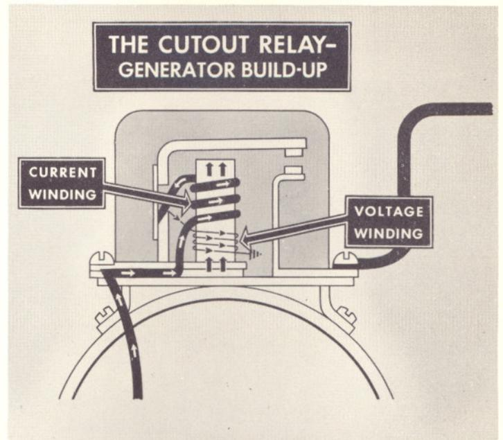
spring tension holding the armature away. The operation of these armatures controls the closing and opening of the charging circuit in the case of the relay, and the addition or removal of resistance in the field circuit in the case of a current or voltage regulator.
