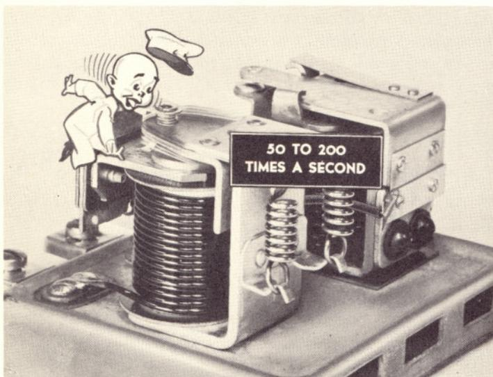
a second, causing a vibrating action of the armature which holds the voltage to a practically constant value. Any winding other than the working winding on a regulator core is used for the purpose of speeding up the rate of armature vibration, thereby reducing the amount of surge when the armature points close.
