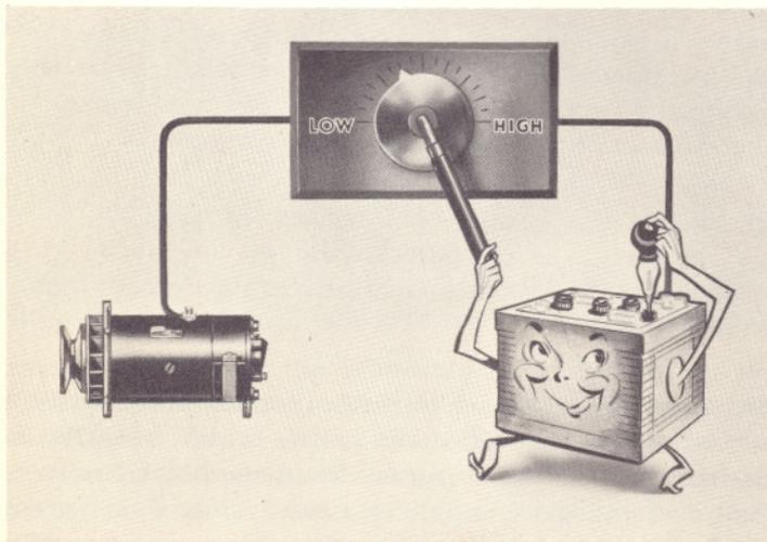
To avoid high voltage and excessive current, the voltage of the charging circuit must be limited as the battery approaches charge. The battery will actually regulate its own charge, within certain temperature limitations, if the voltage in the circuit is kept at a constant value. This
