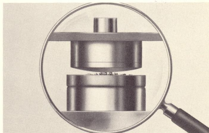
A flat file cannot successfully be used to clean flat contact points. A flat file will not touch the center of the flat point, and will not clean out the slight cavity formed in the point surface in normal operation.
