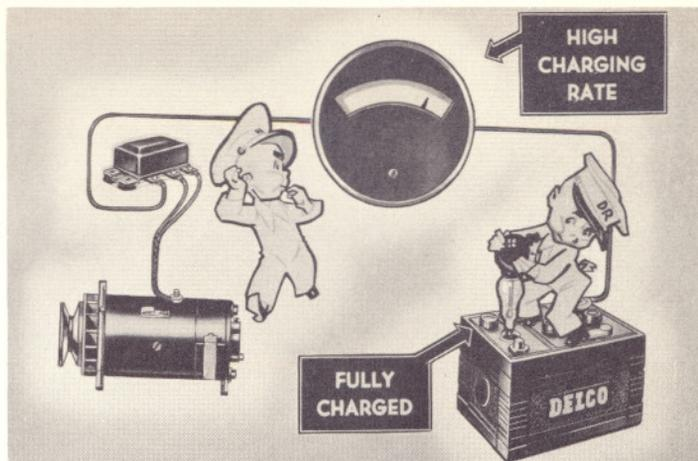
If the output then drops off, the trouble is a grounded field wire between the regulator and the generator. If
