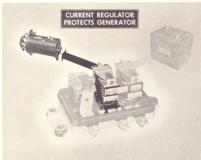
results in a tapering charge rate thus protecting the battery from overcharge and the system from high voltage.
