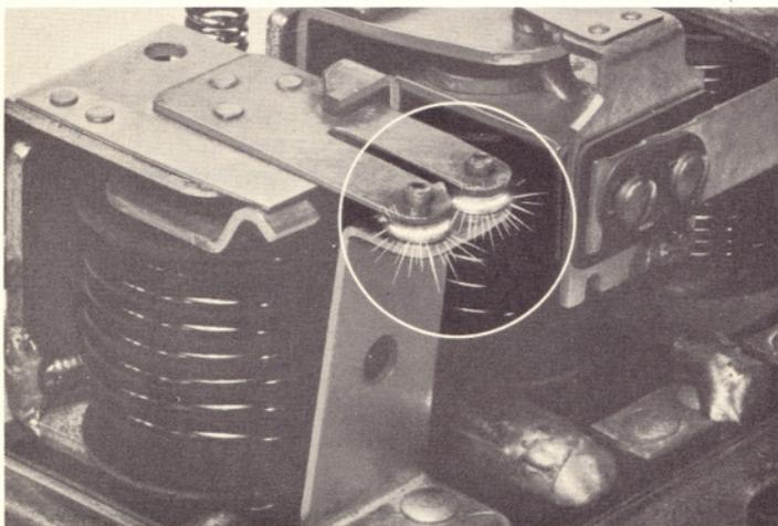
will prevent fluttering, arcing and burning of the cutout relay points which would result if the generator were wrongly polarized with respect to the battery.
