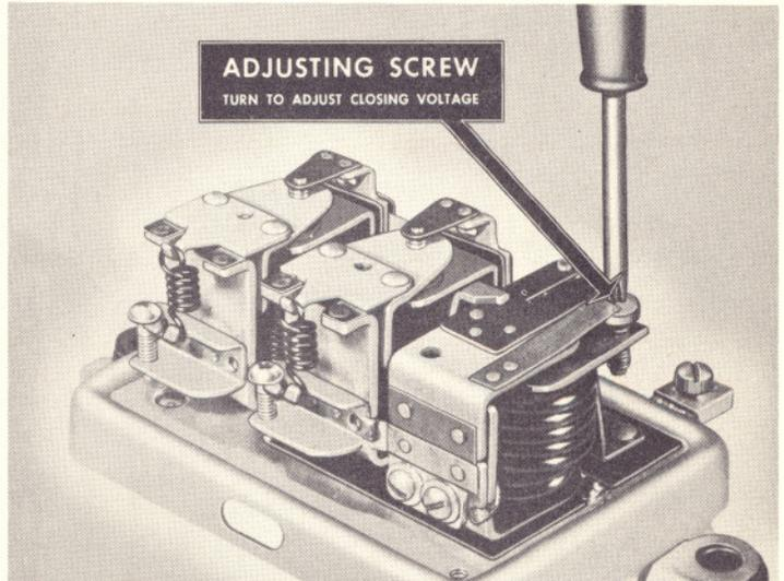
On the 1118300 series of regulators, the closing voltage is adjusted by turning the adjustment screw clockwise to increase spring tension and closing voltage and turning the screw counterclockwise to decrease spring tension and closing voltage. This is a left-hand screw.
