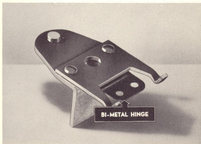
Many current regulators, however, have a bi-metal hinge on the armature for thermostatic temperature control. This permits a somewhat higher generator output when the unit is cold, and causes the output to drop off to a safe maximum as the temperature increases. This is an advantage on short drives where a higher charge rate is obtained for short intervals of time, or until the regulator warms up.
